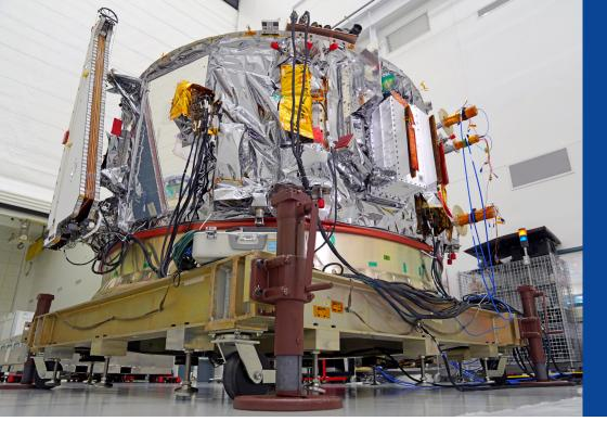
**PIRPL** Prototype InfraRed PayLoad
