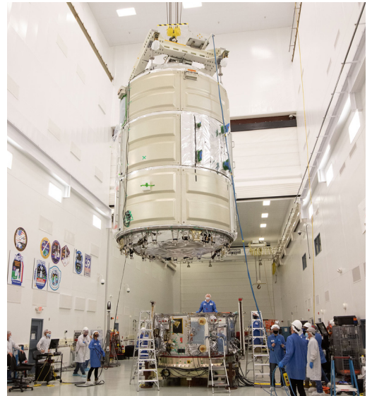
The Cygnus Service Module is mated with the Pressurized Cargo Module at the launch site
