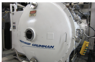
Large vacuum chambers with high capacity vacuum pumping systems able to simulate space and aircraft environments
