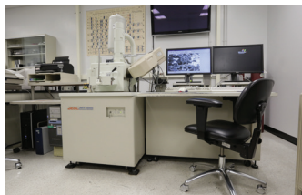
Scanning electron microscope with energy and wavelength dispersive X-ray
